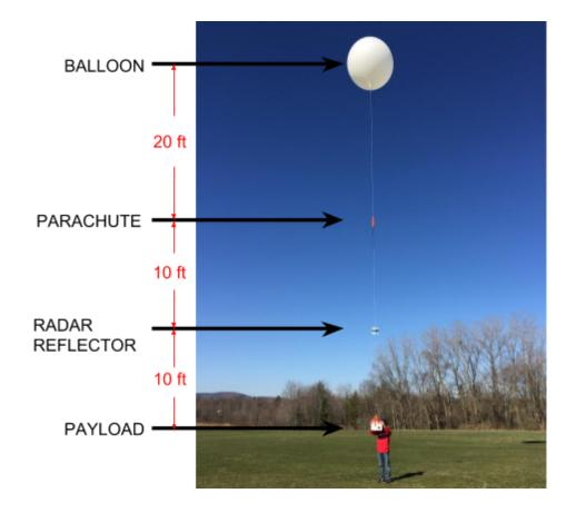
The flight line secures every component (payload box, radar reflector, parachute, balloon) in a different way:
