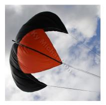
The important specification to keep in mind when buying the parachute is the descent rate. The lighter your payload and the larger the parachute, the slower the payload will fall to the ground. However, the slower the descent rate the further it will travel and descend too fast and you risk damaging the payload and any equipment inside.
