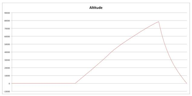
The altitude graph is about as straightforward as it gets. Unfortunately, due to calibration issues, the absolute values are invalid, but the relative height can still be analyzed. Of interest, the rate of ascent looks to be pretty constant, with only one slight change about halfway up. On the descent the rate is decreasing, signifying the work of the parachute and the thickening of the atmosphere.
