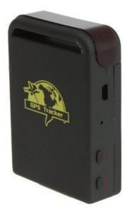
The GSM GPS Tracker was actually meant for tracking cars (read: private investigators). The downside of using this type of tracker is that it will not work without a cell network. So anything above 20,000 ft. is out of question and if the payload lands away from a cell tower, you are out of luck. That being said, as part of a redundancy system and the price (about \$30), it ended up being the perfect backup.
